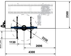
The ECO R. is equipped with a robot inside the cabinet. A universal part table allows rapid part changing, where single parts, as well as several parts, can be inspected at the same time. The table is loaded from the outside of the cabinet either manually or by a second robot to achieve a fully automated system. The ECO R. is available with 160 or 225 kV, and comes with Automatic Defect Recognition (ADR).
