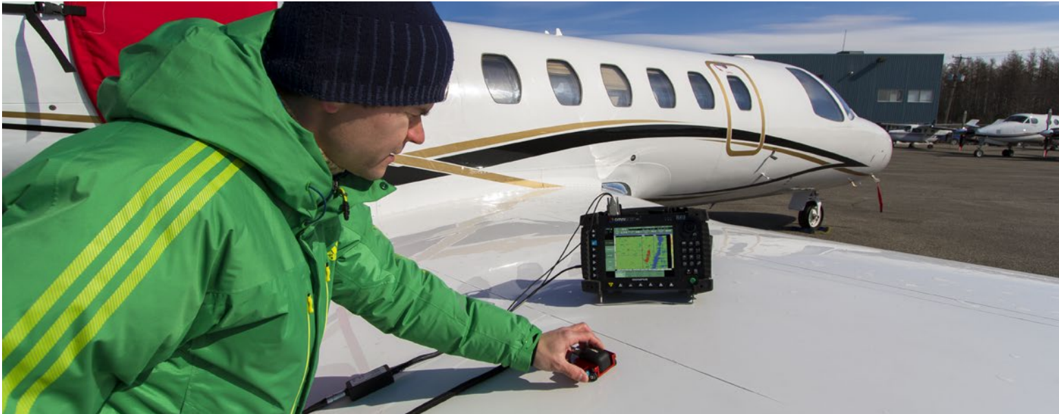
For maximum detection, the MXB software features 8-frequency scanning and amplitude and phase C-scan display.
