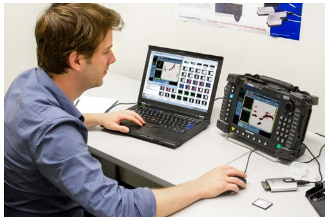
Perform data analysis quickly and efficiently with mouse input. Archive files to a PC with the help of a CompactFlash reader.
